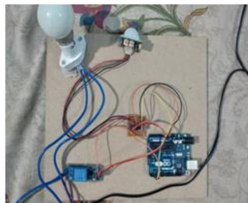
Fig.4. Bulb turns OFF When object leaves out of the room.
